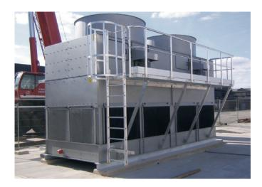
In the wet cooling process, the water to be cooled is sprayed in the air. The air is heated, leading to a chimney effect, and the water gives off its energy. Cooling towers that use wet cooling have a very high power density. The loss of water during evaporation is minimized by droplet separators.
